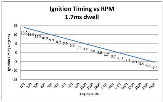
The above chart shows the relationship between ignition timing and RPM with the timer lever in the center or vertical position. At 100 RPM the timing is 14° advanced and at 2000 RPM the timing is retarded 5.4°. This is why the timer lever needs to be pulled back when starting the engine and pushed forward when running at higher RPM.
