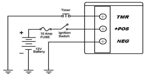
When wiring the input connections use at least 14ga stranded wire, 10 amp fuse, and ignition switch. It is a negative ground system so grounding is very important. It is recommended to make sure the aluminum case, negative terminal connection, engine, and battery have good chassis ground connections.
