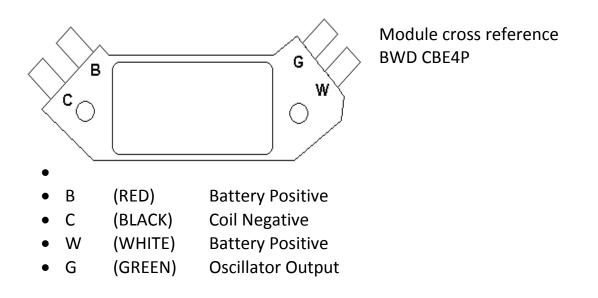
To replace module the tools required are a #2 phillips, 11/32 socket, and a small needle nose pliers. Carefully remove the 4 wires by holding the body of each crimp connector with the needle nose pliers and sliding it away from the module. Do not pull on the wire as it may come out of the crimp connector. Remove hardware and module.
